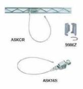
Grounding Cable: ASK16S or ASKCR provides an effective method of electrostatic discharge for any Metro wire shelf unit (stationary or mobile) when used in conjunction with conductive split sleeves. The drag cables ensure a conductive path to ground when used with ESD flooring.
